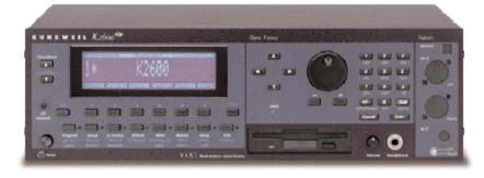
another section of battery protected RAM. A standard K2600 arrives with 465kB of PRAM - reasonable compared to the K2500's 256kB and generous compared to the K2000's piffling 120kB. With 456kB you won't be immediately rushing out for an upgrade. The K2600's program storing capacity can expanded to 1.5MB, a 256kB improvement on the K2500's capacity. Of course the K2600, like its predecessors, will accept sampling RAM. The 72-pin SIMMs are still the order of the day, but 128MB is still the limit.
